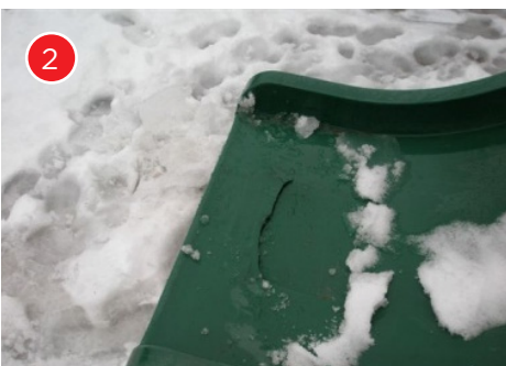
This tear could be an entanglement hazard.
