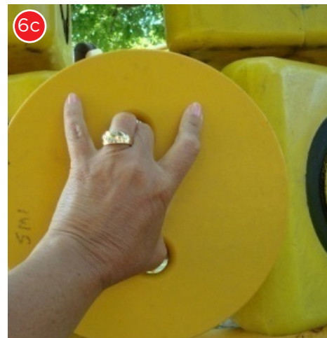
The head probe does not freely enter; therefore, this tic-tac-toe panel poses a head entrapment hazard and should be corrected.
